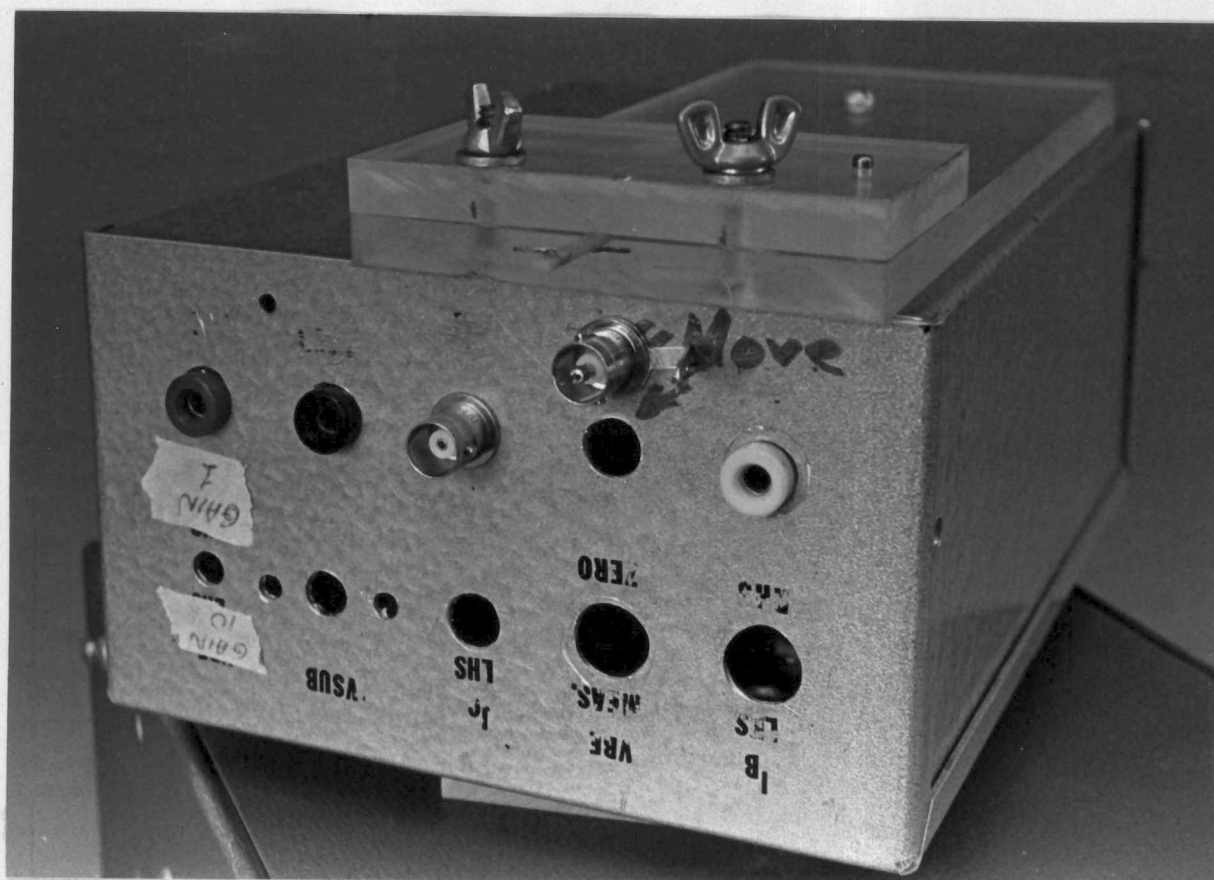
Figure 13. Photograph of the Clamp Mounted on the Amplifier.
