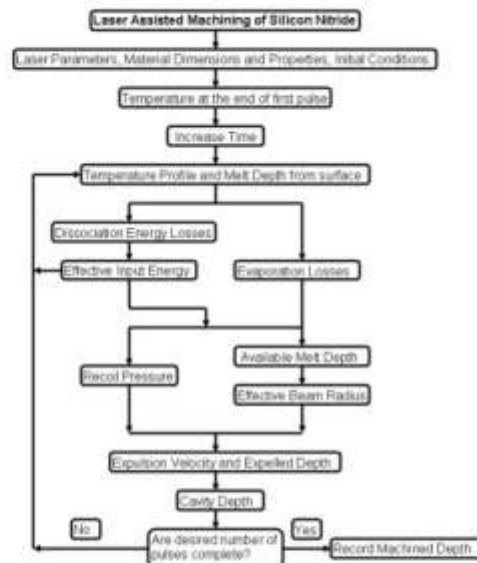
Fig. 3. Stepwise procedure for machined cavity depth prediction.
