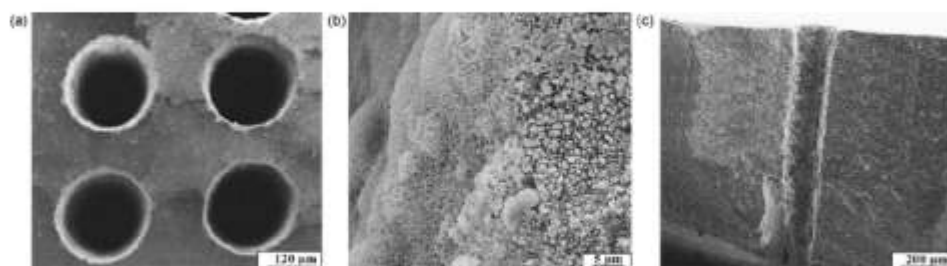
Fig. 22. Holes drilled on pelcast green body of alumina. (a) Top view, (b) hole edge, (c) cross-section of hole. (After Guo et al. 97 with permission. Copyright Elsevier.)
