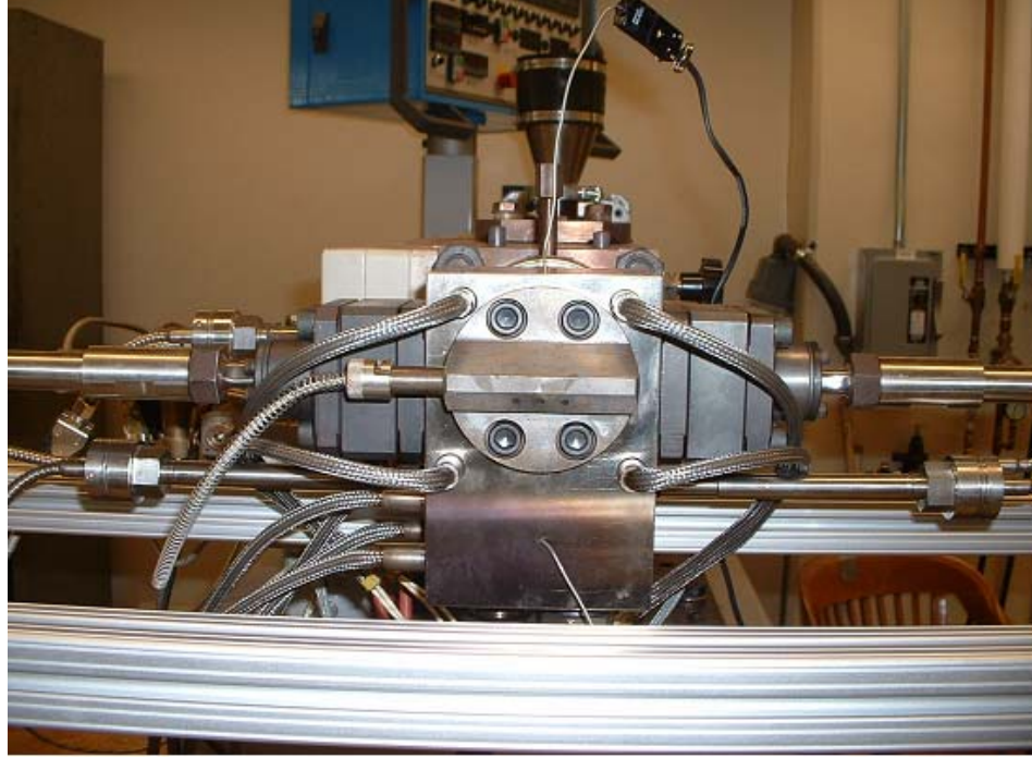
Figure 2.2-2: Picture of the Online Rheological Sensor mounted on the Leistritz twin-screw extruder (photo by Larry Spencer)
