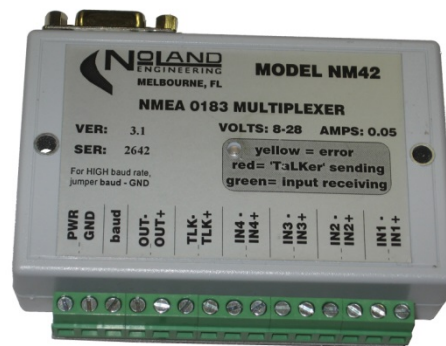
Figure 4.2. The NMEA 0183 multiplexer used to combine distance sensor output and GPS data into a single data string ( http://nolandeng.com/nm42.php , accessed May 2014).
