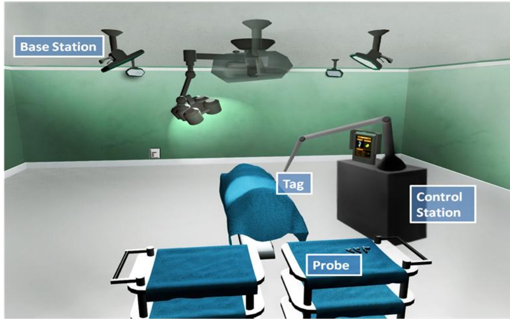
Figure 10: Microwave positioning subsystem overview showing major components: control station, base station, probe, and tag
