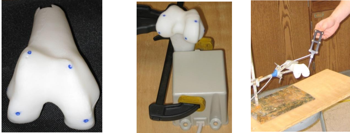
Figure 14: a) Synthetic Femur with machined landmark recesses b) Synthetic femur mounted to EM transmitter c) Femur mounted for static optical experiment
