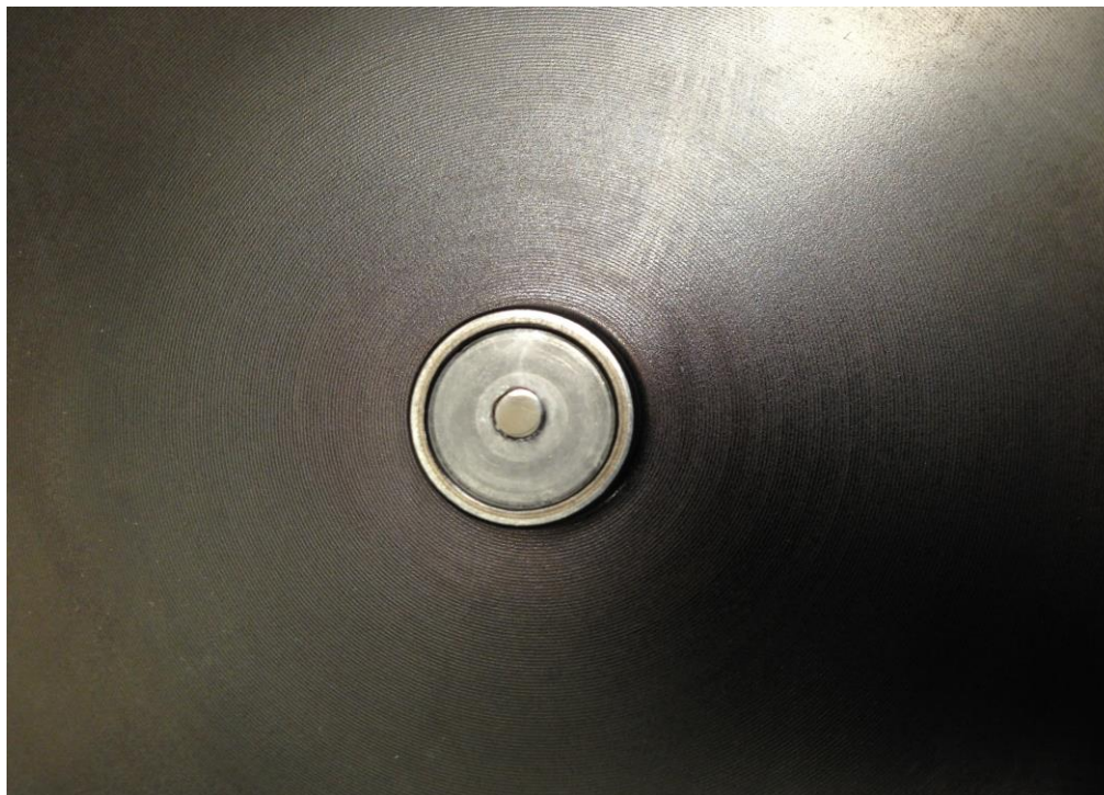
Figure 3-10 Cu based BMG 3 mm disc specimen secured in the top holder device.
