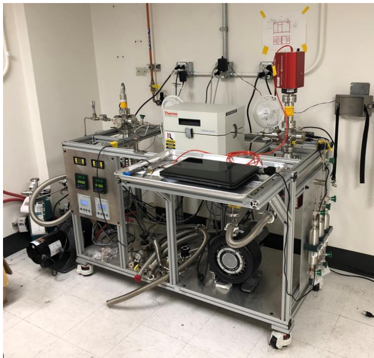
Figure 3-47 TDS equipment located in LAMDA at ORNL.
