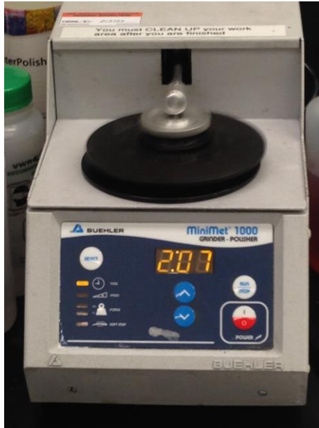
Figure 3-9 Left) Buehler MiniMet 1000 semi-automatic grinder/polisher. Right) Adjustable sample holder which allows for grinding of sample to a precision of tens of microns.
