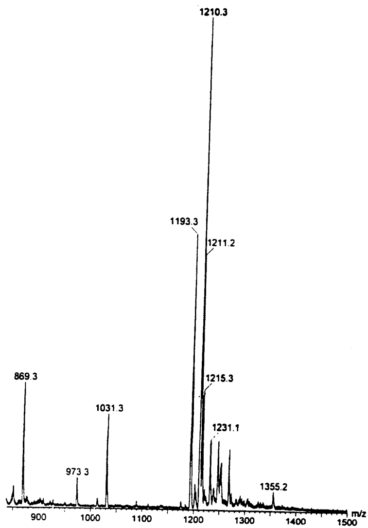
Figure 17. The CM- \beta -CD ammonium adduct obtained at 50 V.
