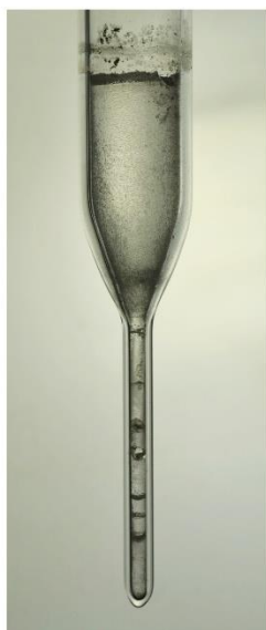
Figure 70. Photographs of backlit 12 mm diameter mixed \text{Cs}_2\text{ZnCl}_{4-x}\text{Br}_x crystals inside ampoules, as well as several cut and polished slices.
