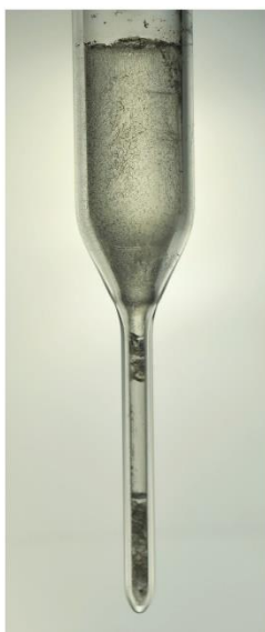
Figure 70. Photographs of backlit 12 mm diameter mixed \text{Cs}_2\text{ZnCl}_{4-x}\text{Br}_x crystals inside ampoules, as well as several cut and polished slices.
