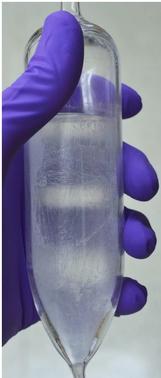
Figure 43. Photograph of as-grown 38 mm diameter \text{Cs}_2\text{ZnCl}_4 crystal inside the growth ampoule.
