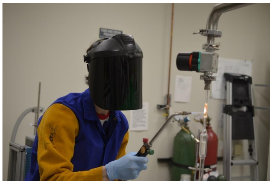
Figure 9. Photograph of PhD student Daniel Rutstrom sealing a quartz growth ampoule with an oxy-hydrogen torch.
