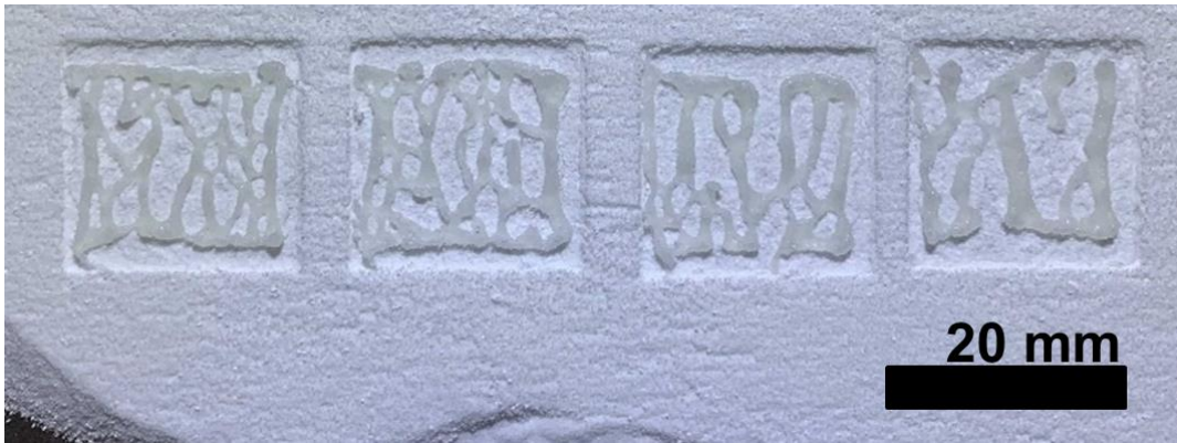
Figure 25. Single layer scans of the 12k sample resulted in ribbed structures, which did not accurately match the set layer geometry.
