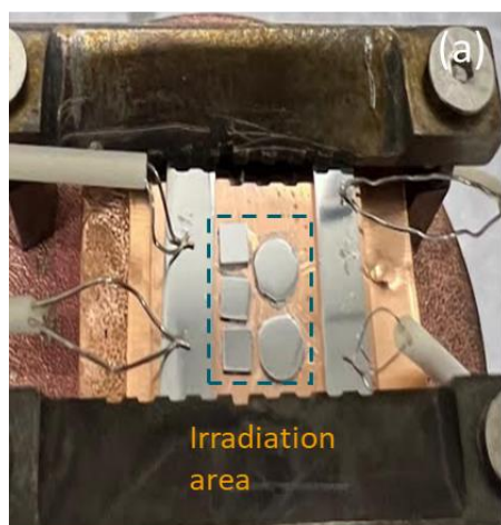
Figure 3.3 (a) specimens loaded on the stage for irradiations. (b) SRIM prediction of the depth-dependent displacement damage and injected ion concentrations of pure Fe irradiated by 8 MeV Fe ions to mid-range doses of 0.1, 0.2 and 0.6 dpa.
