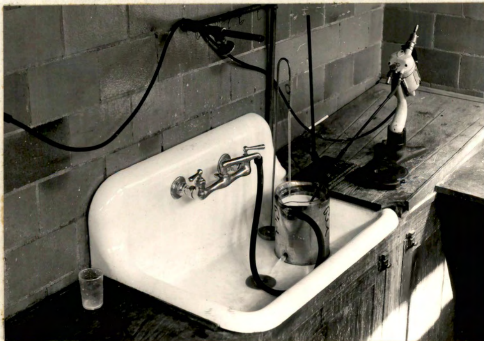
Figure 11. Pasteurizing two-quart samples. The hot water from the tap is forced through the rubber tube into a copper tube which circles a glass beaker filled with milk. Holes in the copper tube allow the hot water to spray on the sides of the beaker and heat the milk. The milk is stirred with a glass rod connected to an electric motor to maintain a uniform temperature throughout.
