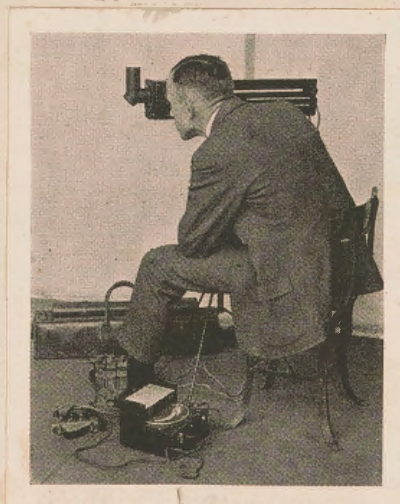
READING ILLUMINATION ON THE HORIZONTAL PLANE WITH THE SHARP-MILLAR PHOTOMETER.
