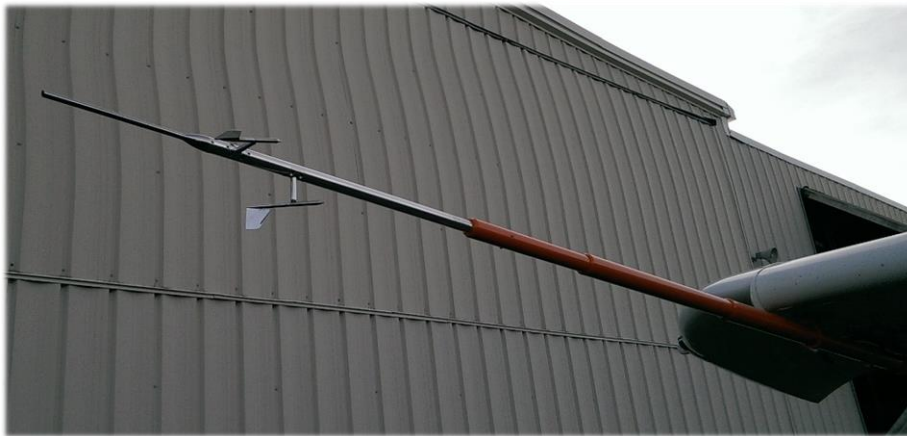
Figure 1: NASA Air Data Boom Design with Flow Angle Vanes on the UTSI Cessna 210 right wingtip.
