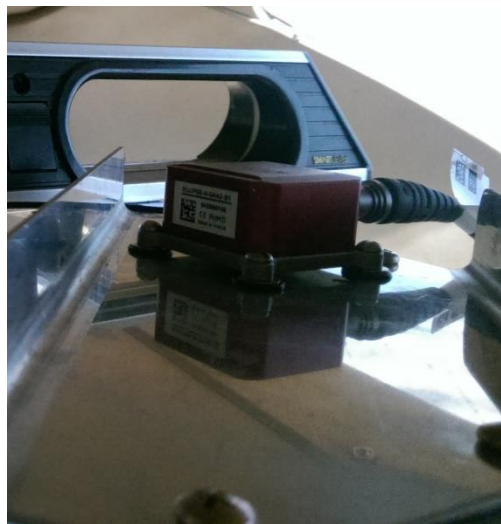
Figure 16: Ellipse-N INS Installed in Cessna 210 DAS Rack in Rear Seat Station
