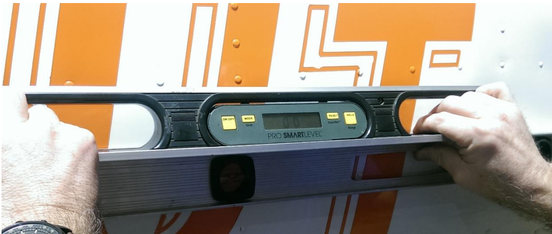
Figure 13: Aircraft water level reference line. The ADS Boom aligned with this reference line; the INS unit has a 0.1^\circ offset from this reference line.
