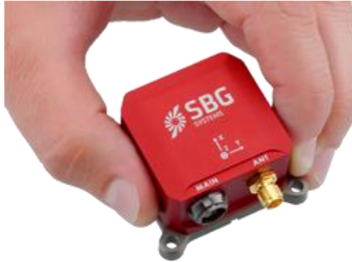
Figure 27: SBG Ellipse-N INS Unit
