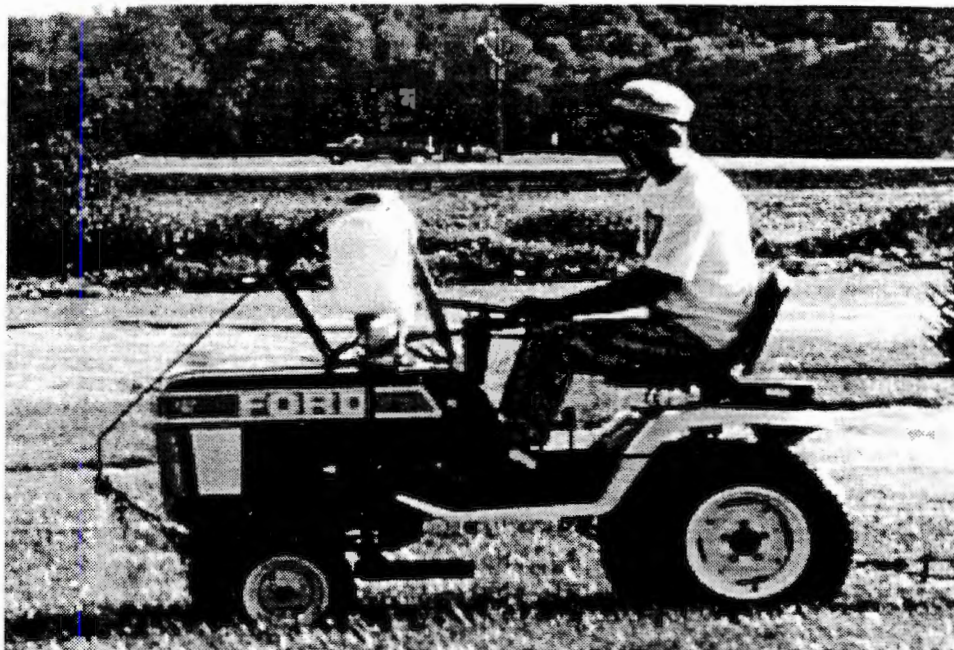
Figure 4: Ford LGT 14 with backpack sprayer mounted on the hood for applying free surface moisture to the turf just ahead of the front wheels.
