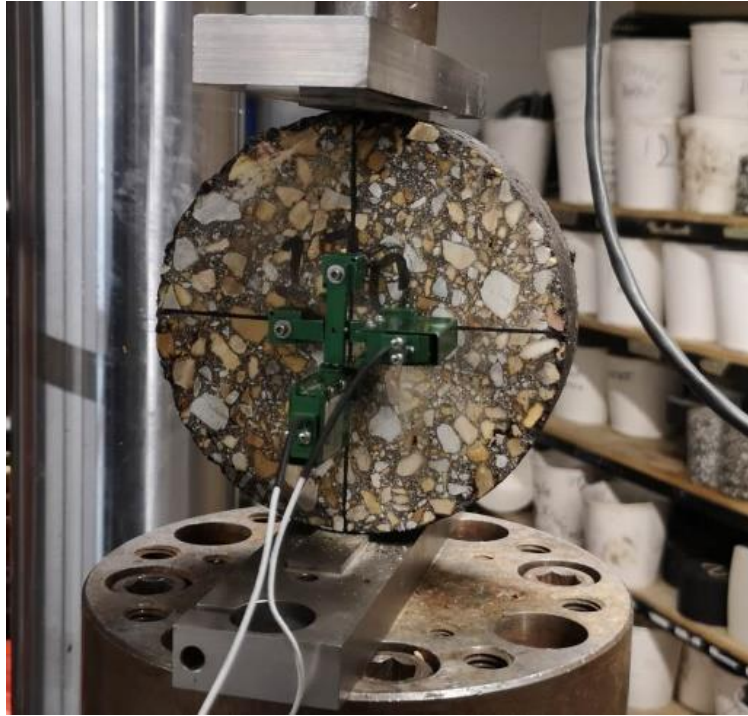
Figure 4-3. Superpave IDT test setup.
