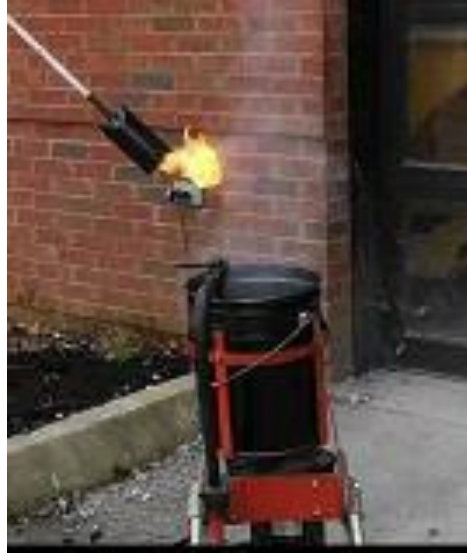
Figure 5-7. The fire heating simulation using torch blow test.
