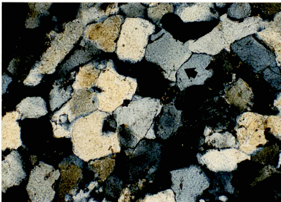
Figure 5.7. Thin-section photomicrograph, under cross-polarized light, of sample FG-1 from Flat Gap, TN (Locality FG in Figure 1.2) illustrating pressure-solution features such as concave/convex grain boundaries (arrow) and quartz overgrowths. Such features are common to the FGB variant and in the associated pebble lags. Field of view is 2.3 mm in the long dimension.
