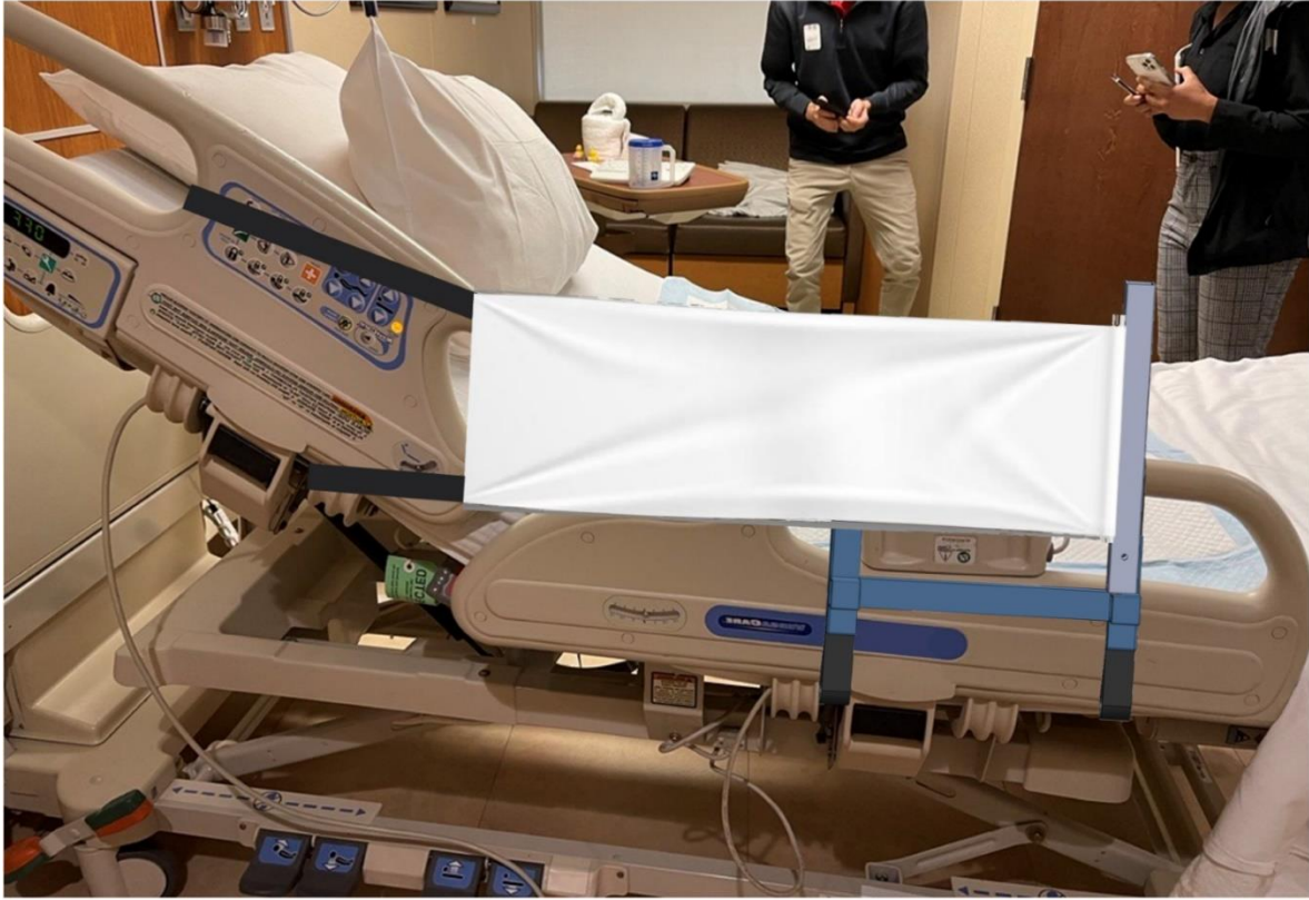
Figure 5: Rendering of the CRIB Device Assembly in the Hospital
