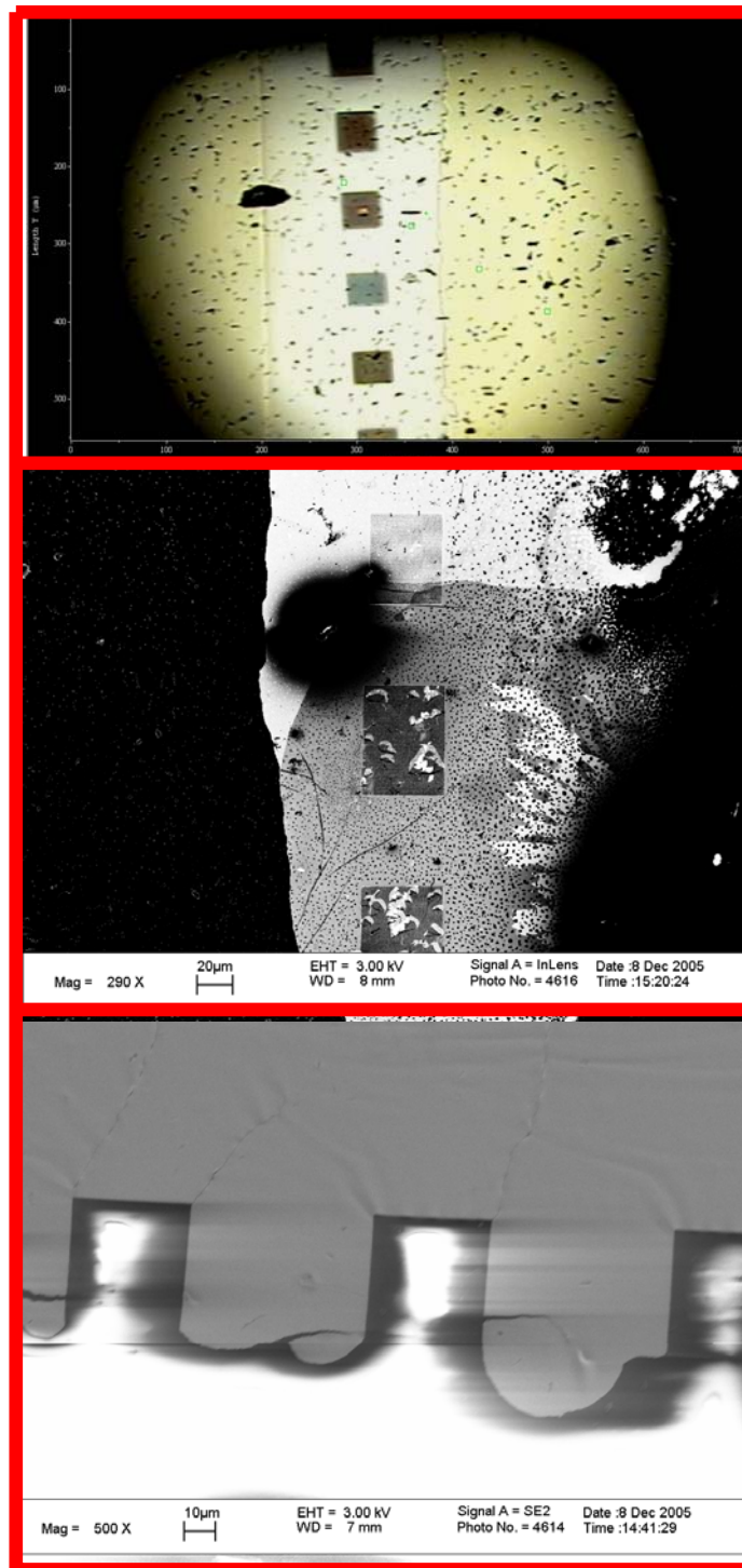
Figure 3.10 (Top) Shows the white light illumination of the stamp after depositing Cal[4] and before the transfer process. (Middle) Shows SEM image of stamp after the transfer process. (Bottom) Shows SEM image of PMDS after nTP.
