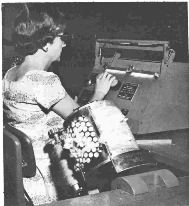
Developing Cotton Fiber Testing Machines: This Physics Department laboratory worker is brushing a pair of cotton samples on the Digital Fibrograph. The samples were taken with the Fibro-sampler shown in the foreground.
