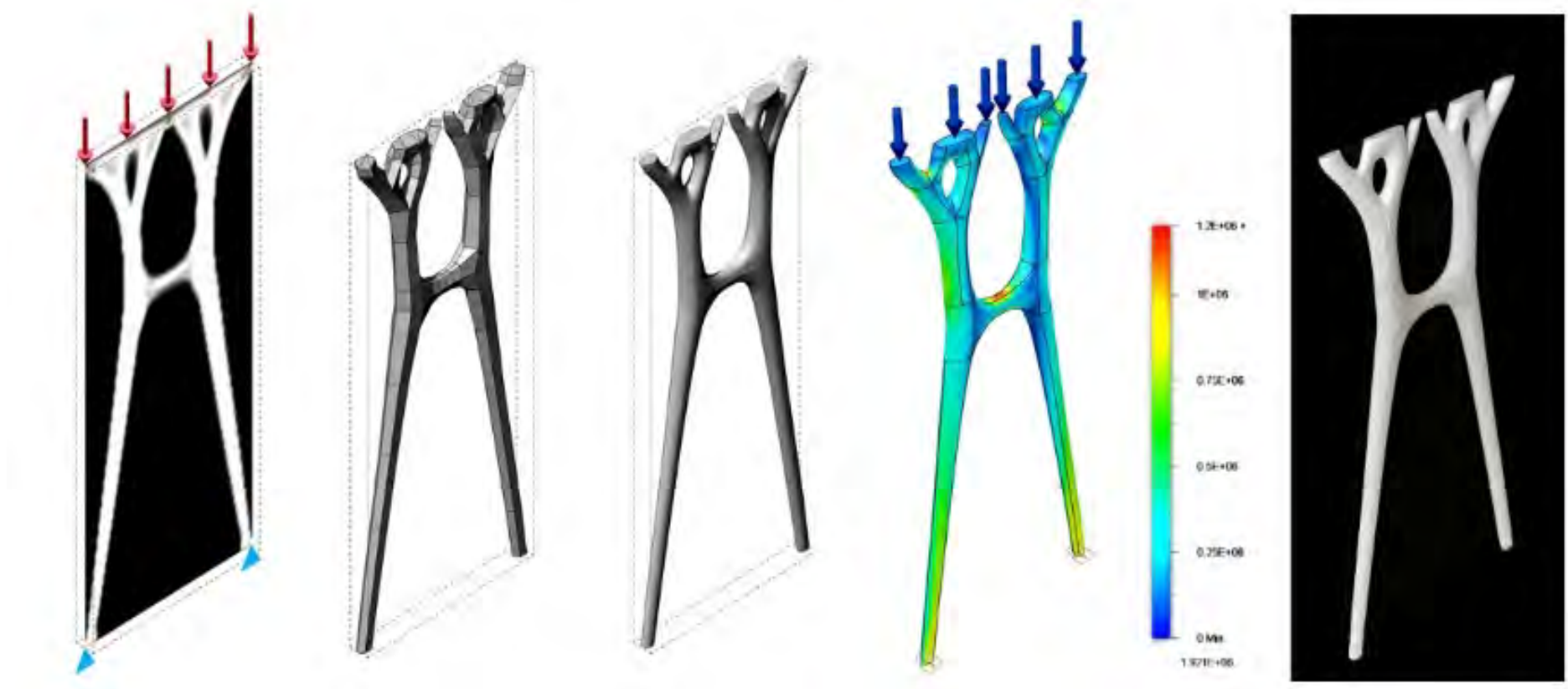
Results for topologically optimized wall (stiffness mesh, low polygon mesh, smoothed mesh, finite element stress analysis, 3D print) (fig. 5)
