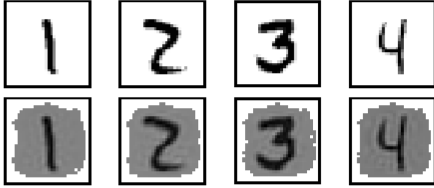
Figure 5.6: Original MNIST handwritten digits (top) and the reconstructed PCA reduced digits (bottom)
