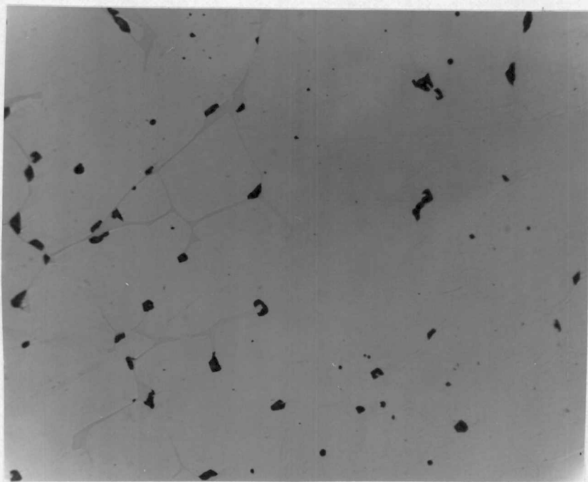
Figure 56. High ferrite (FN \approx 8) CF3 alloy in the as-cast condition, as EPR tested. 250 X.
