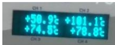
Fig. 5-94. Temperature reading of GaN devices of the PFC stage without good thermal contact. Ch1: top A top source; Ch2: bottom B source; Ch3: top B source; Ch4: bottom B drain.
