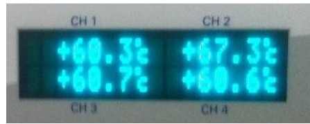
Fig. 5-95. Temperature reading of GaN devices of the PFC stage with good thermal contact. Ch1: top A top source; Ch2: bottom B source; Ch3: top B source; Ch4: bottom B drain.
