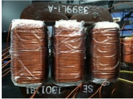
Fig. 3-12. A prototype of the three-limb three-phase zigzag transformer.
