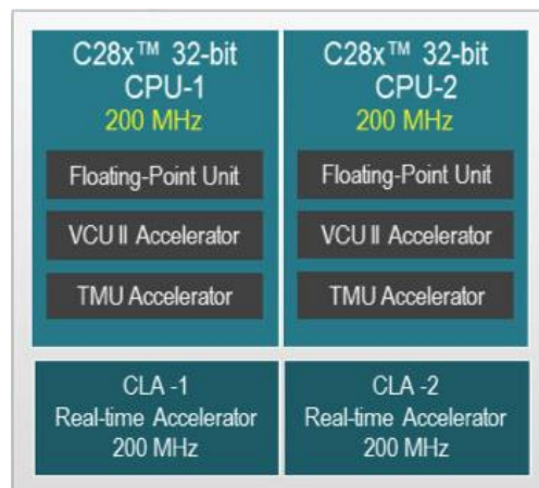
Fig. 5-78. The computation units inside TMS320F28377D [336].
