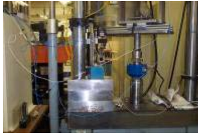
Figure 32. Extensiometer and Load Cell on Test Setup
