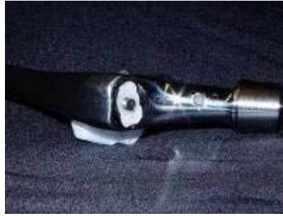
Figure 21. Mounting Stud Placement on Femoral Stem
