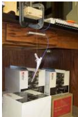
Figure 26. A.) Resonant Test for Femoral Stem B.) Resonant Test for Femoral Stem with Head
