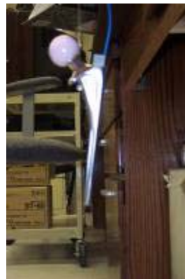
Figure 26. A.) Resonant Test for Femoral Stem B.) Resonant Test for Femoral Stem with Head
