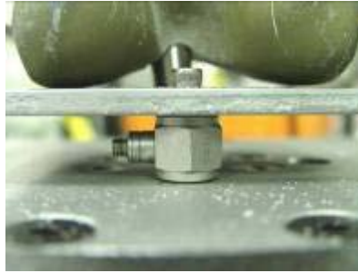
Figure 24. Femur Mounted on Force Transducer
