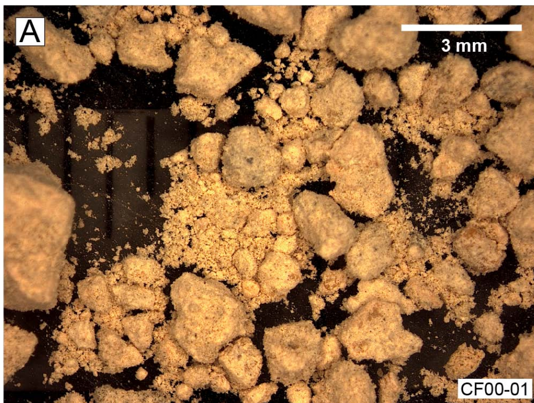
Figure A1.1. Photograph of caliche aggregates.
