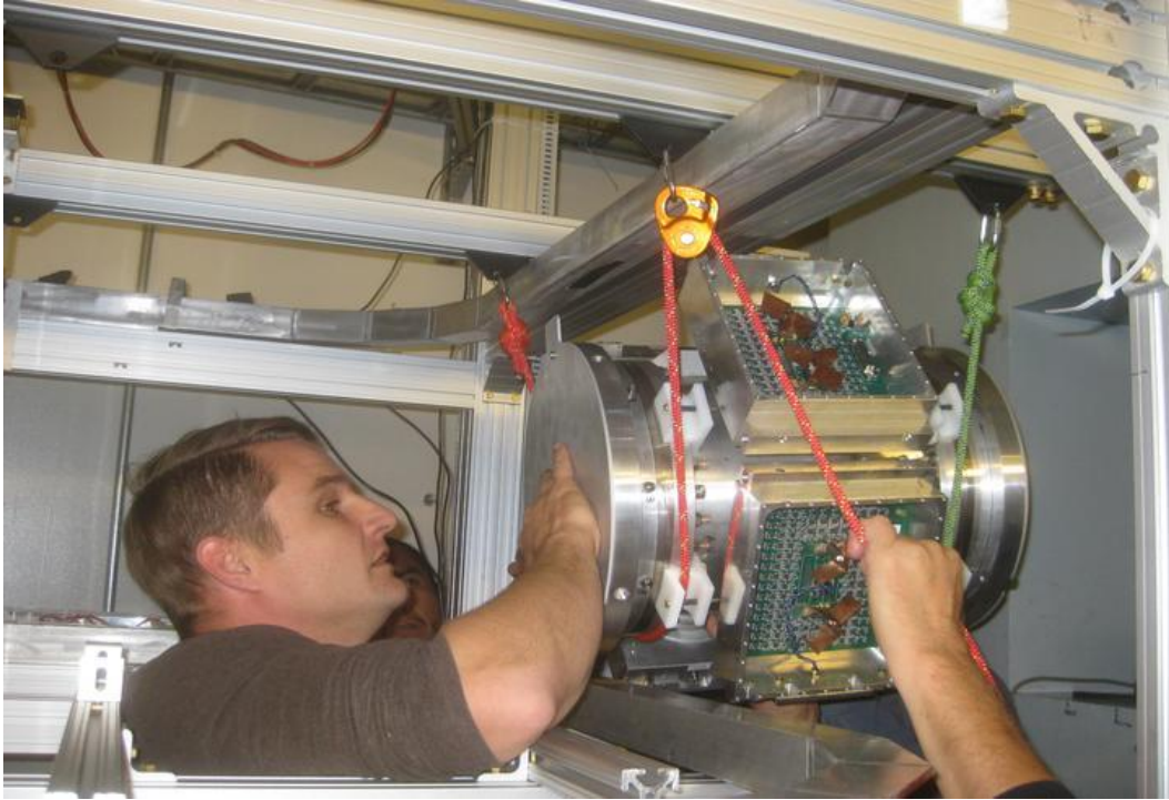
Figure 33. The ion chamber being hoisted into place. Note the progress capture pulley (orange). Photo courtesy of Jack Thomison.
