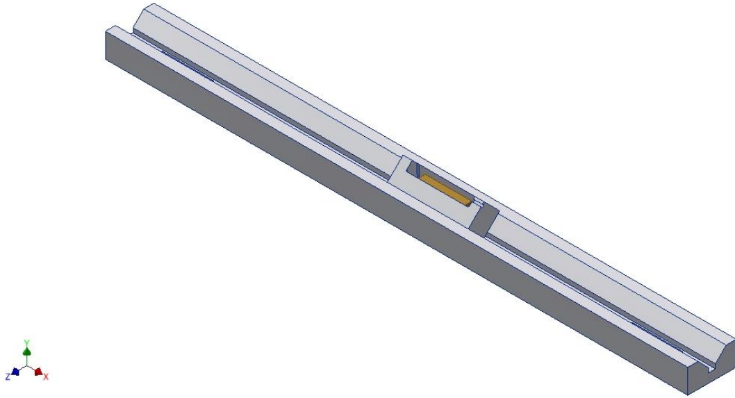
Figure 12. The magnetometer and sled placed into the matching groove in V-block.
