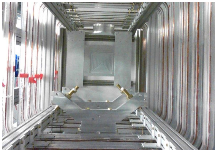
Figure 32. The four-jaw collimator installed in front of the spin rotator. The ion chamber mount is visible in the foreground.
