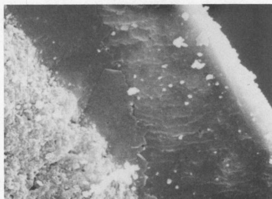
Fig. 4.16. Secondary electron micrographs of SiC fracture surfaces — 100% Ar diluent (a,b) Run 92, T = 1280 K, (c) Run 84, T = 1180 K, (d) Run 84, T = 1180 K, annealed 1180 K, and (e,f) Run 45, T = 1073 K.
