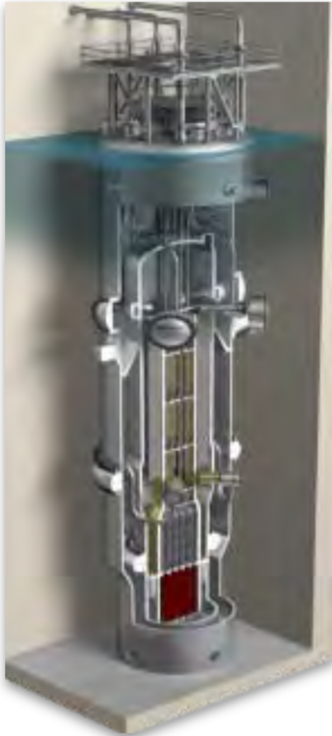
Figure 1.3: Cutaway diagram of the NuScale module situated in its pool [5].
