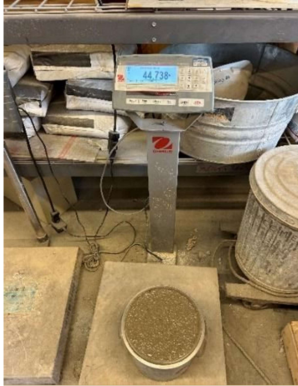
Figure 3-11 Unit weight measurement using super air meter bowl
