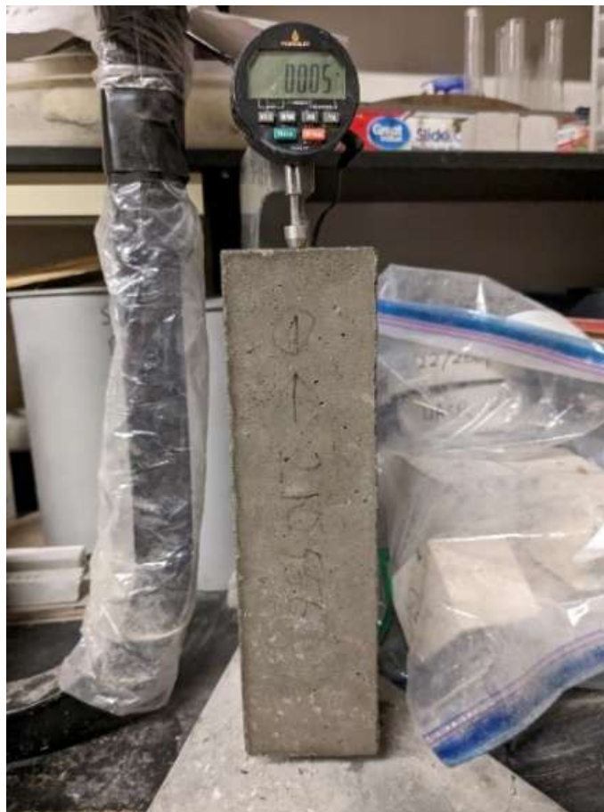
Figure 3-17 Shrinkage beam placed into a comparator
