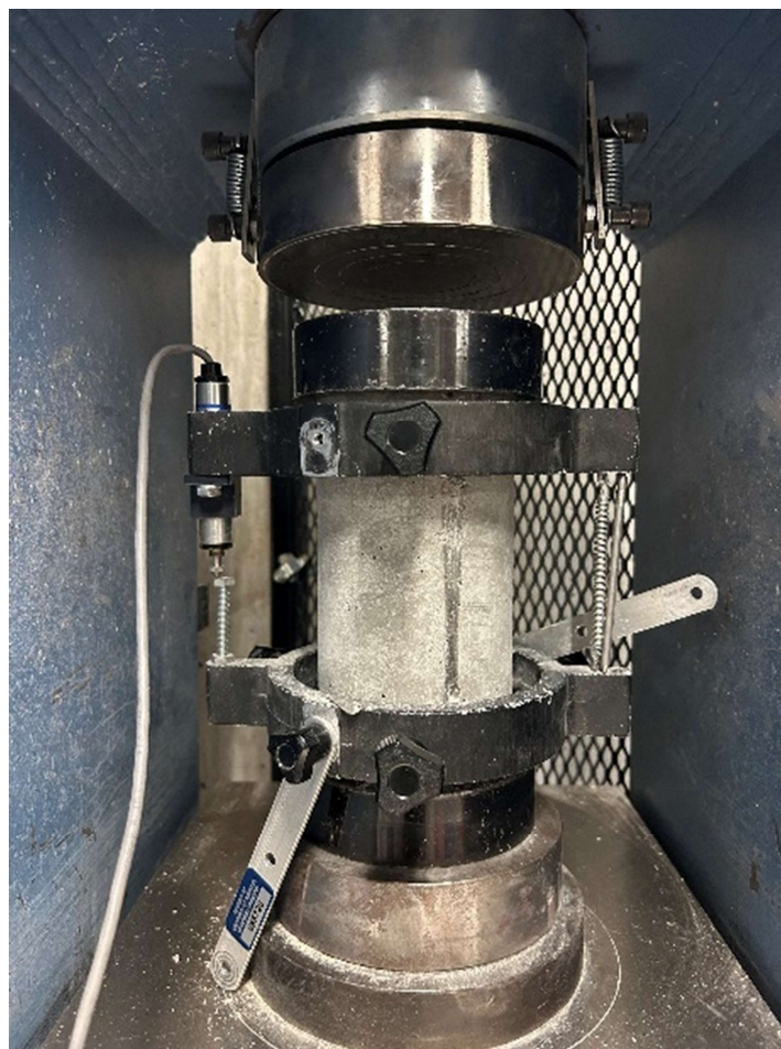
Figure 3-16 Modulus of Elasticity test setup
