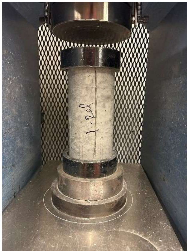
Figure 3-15 Compressive strength test setup
