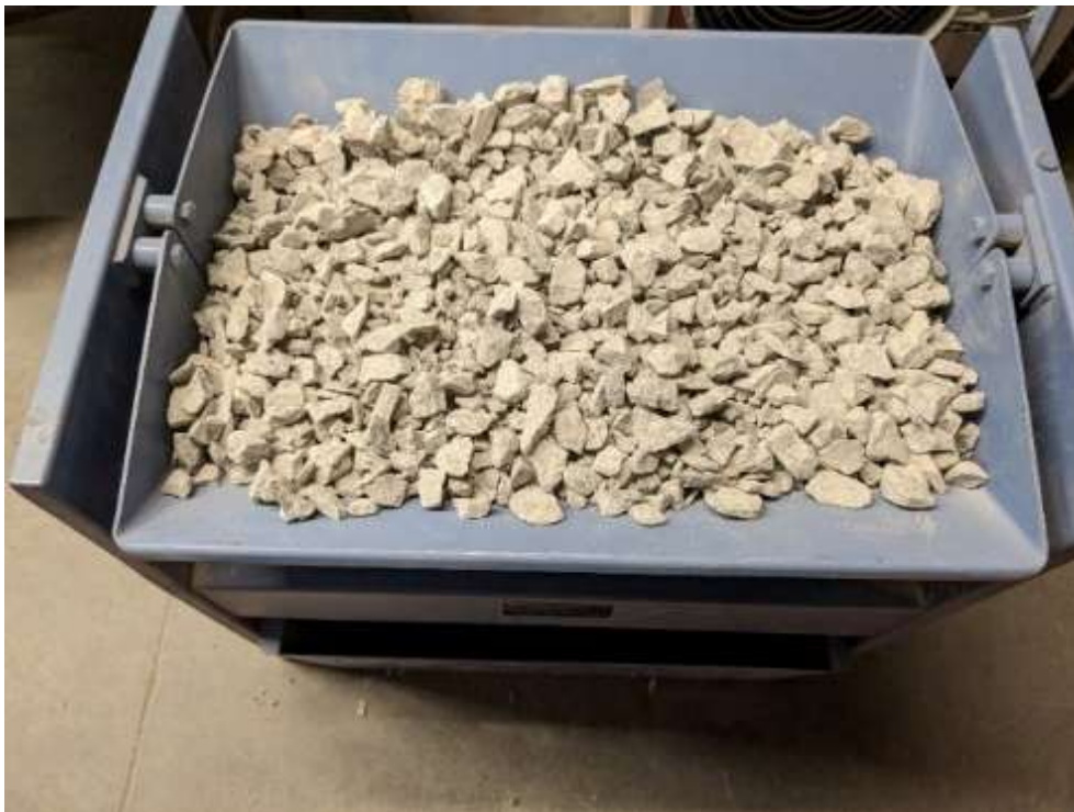
Figure 3-7 Use of splitter to collect representative sample
