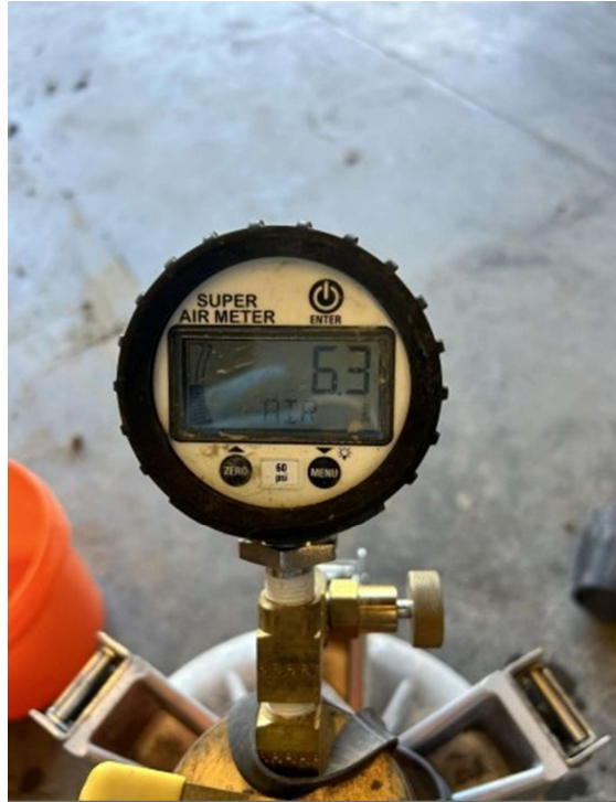
Figure 3-12 Air content testing using the super air meter
