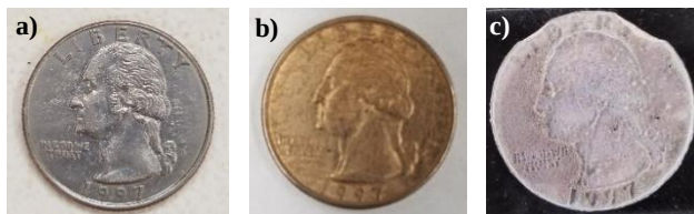
Figure 3.5 Producing conformal polyethylene films using precatalyst 20 and light-activated olefin polymerization. The pictures shown are of a U.S. quarter a) after deposition and evaporation of the precatalyst 20/I-PAG solution, b) after UV exposure, and c) after the film is lifted from the support via submerging in methanol.
