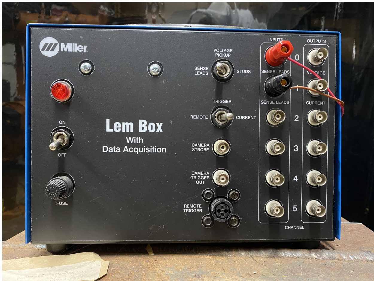
Figure 4.3: LEM Box voltage and current sensor
