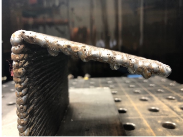
(b) Side view of a 105° WAAM overhang
