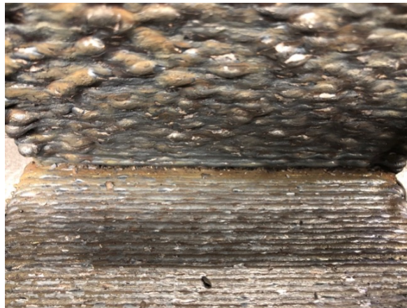
(c) Underside of the NGA portion of a 105° WAAM overhang
