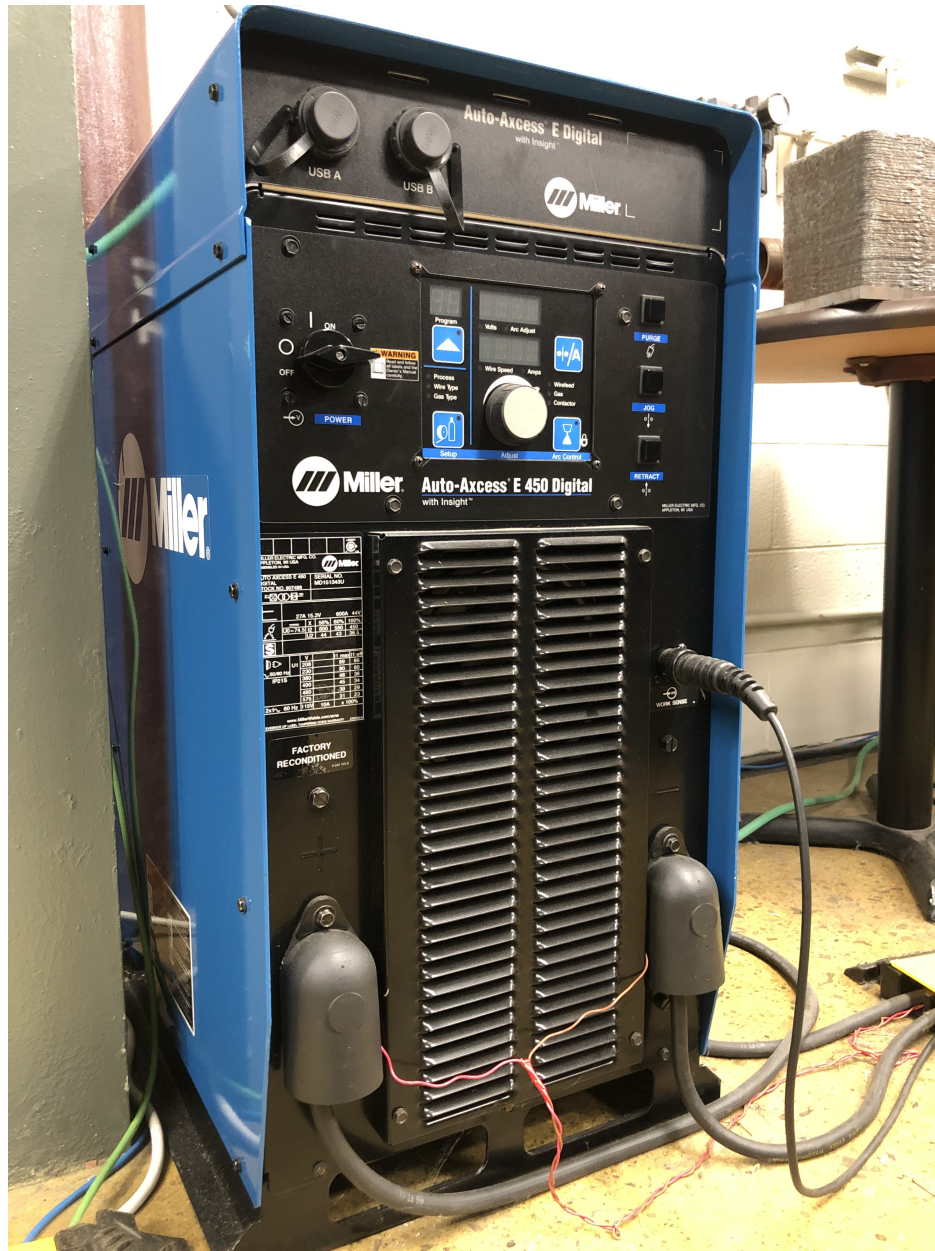
Figure 1.4: Miller AutoAxcess E450 Gas Metal Arc Welding power supply
