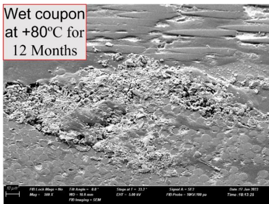
Figure 90: Effect of temeprature upon the matrix in the dry and wet temperature conditioned coupons
