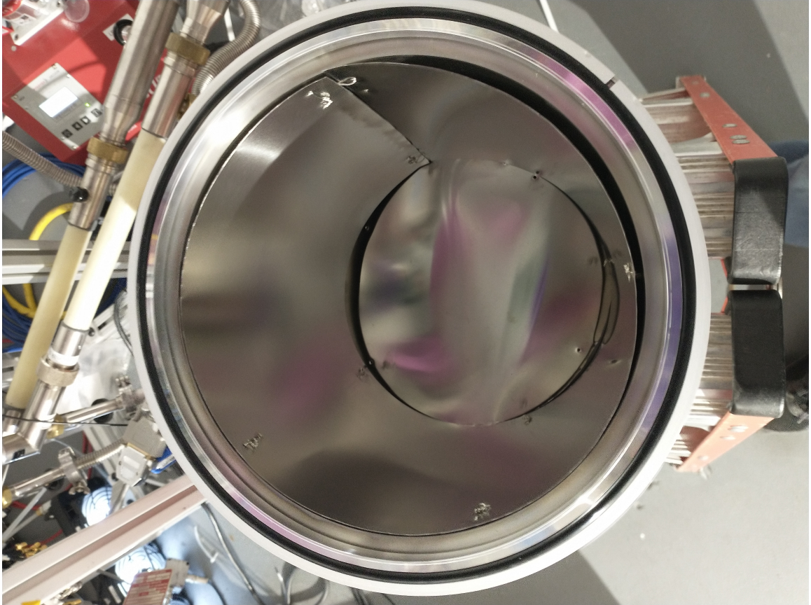
Figure 5.6: This is the thermal radiation shield that was implemented in the Mini-Chamber during the initial thermal profile measurement.
