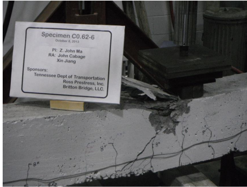
Figure 3.46 – Failure Mode of Specimen C0.62-6
