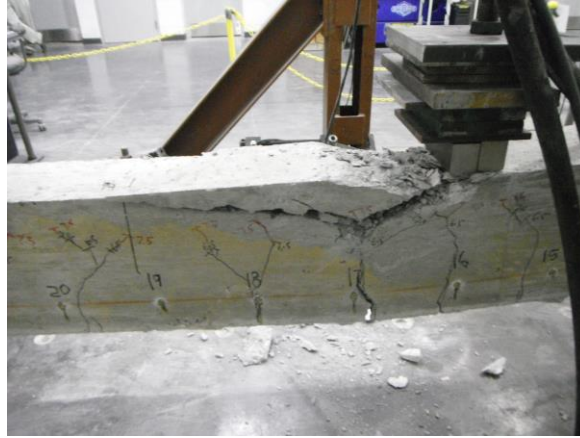
Figure 3.16 – Failure Cracking of Specimen A0.70-6 at Load Point
