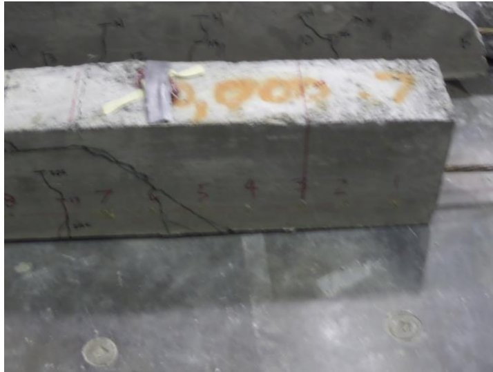
Figure 3.37 – Failure Mode of Specimen A0.70-10
