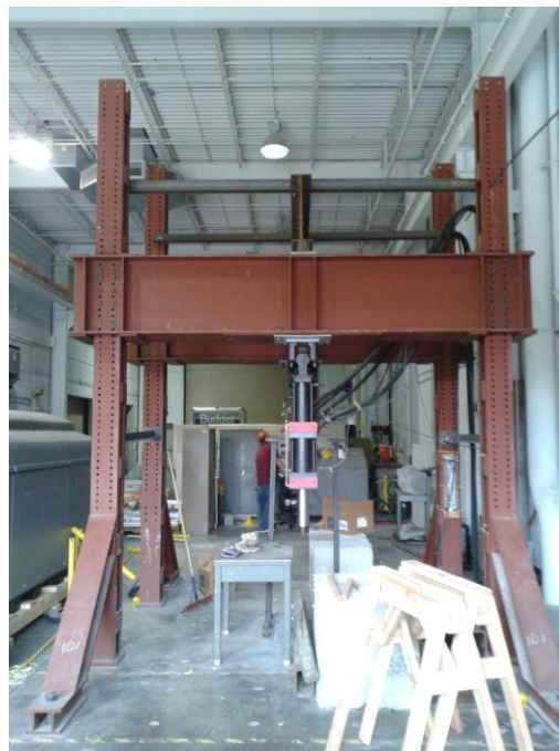
Figure 3.5 – Load Frames with MTS Actuators at NTRC
