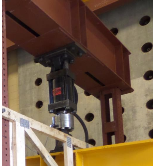
Figure 4.14 – 150 kip Actuator with Load Cell Underneath
