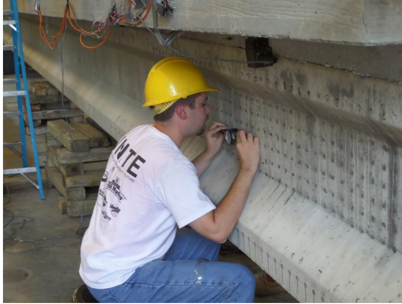
Figure 4.22 – DEMEC Gauge Pattern and Measurement between Points
