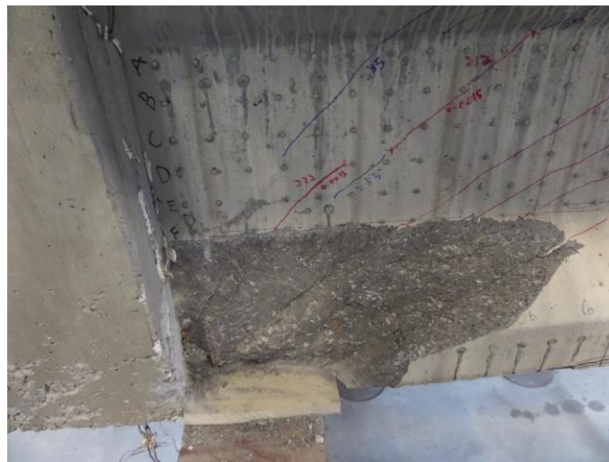
Figure 4.34 – Shearing of Bottom Flange at Final Loading, Specimen 0.70B
