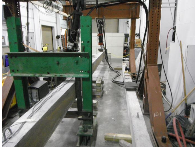
Figure 3.8 – Side Bracing Frame and Cribbing
