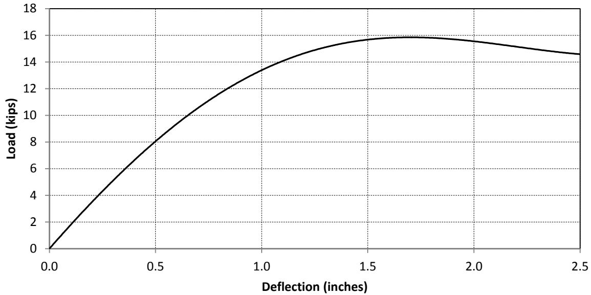
Figure 3.50 - Load versus Deflection at Load Point, Specimen A0.62-8
