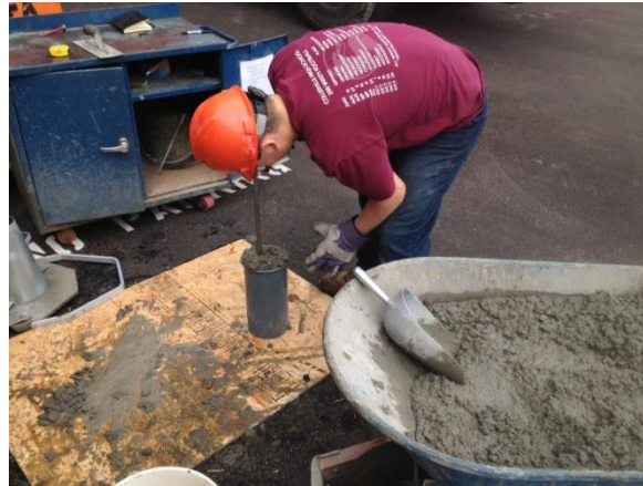
Figure 4.6 – Cylinder Preparation and Concrete Property Measurement at Placement
