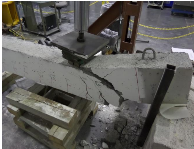
Figure 3.49 – Failure Mode of Specimen A0.62-8
