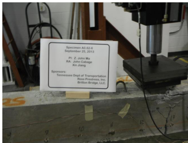
Figure 3.43 – Failure Mode of Specimen A0.62-6
