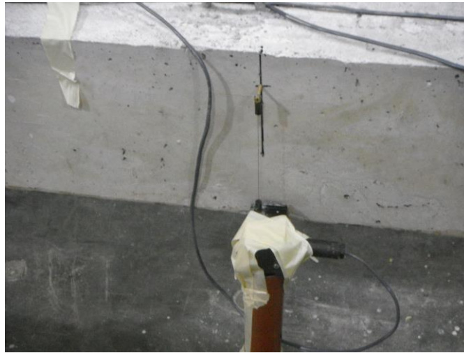
Figure 3.10 – Vertical Displacement String Potentiometer Attachment
