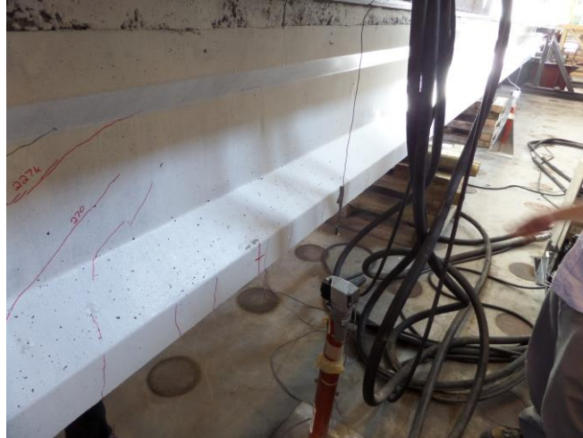
Figure 4.11 – String Potentiometer used in Measuring Beam during Testing
