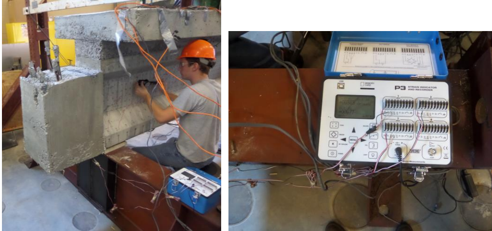
Figure 4.17 – Strand Slip Measurement for Second Full-Scale Test
