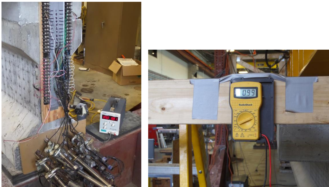
Figure 4.16 – LVDTs used for Strand Slip Monitoring
