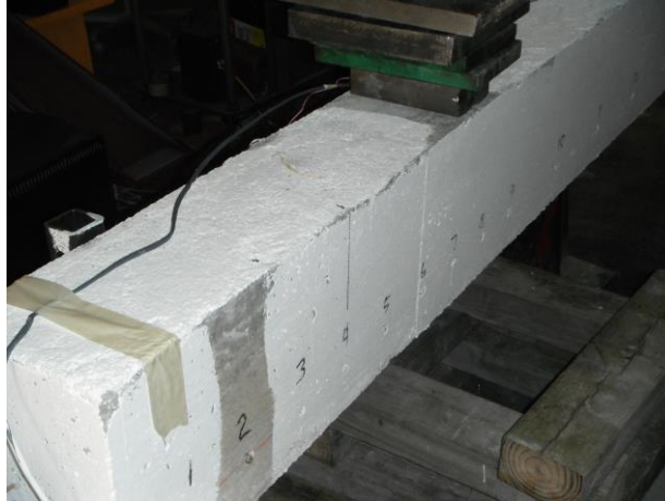
Figure 3.3 – Typical DEMEC Gauge Point Layout
