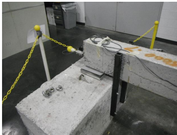
Figure 3.7 – Live End of Development Length Testing Specimen
