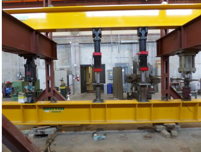
Figure 4.10 – Series of Actuators to Test Beam Specimens
