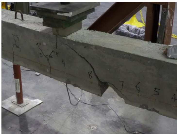
Figure 3.52 - Failure Mode of Specimen A0.62-8
