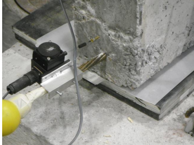
Figure 3.2 – String Potentiometer Positioned at the End of the Extended Strand
