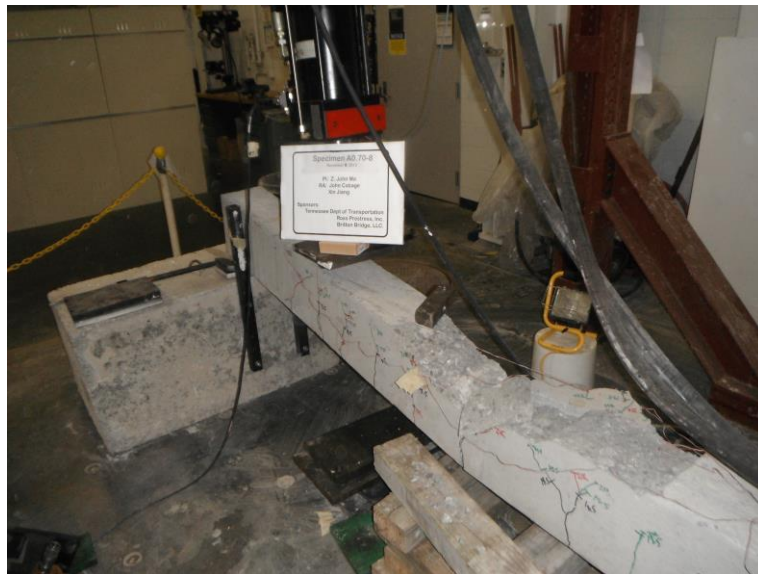
Figure 3.31 – Failure Mode of Specimen A0.70-8
