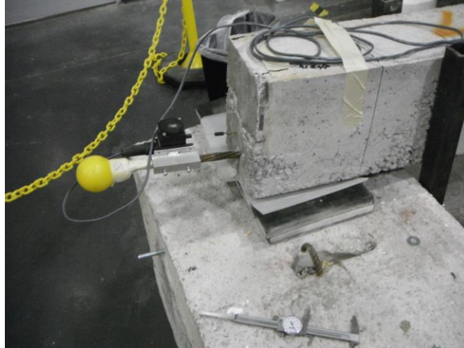
Figure 3.11 – Strand Slip Monitoring String Potentiometer at Beam Live End
