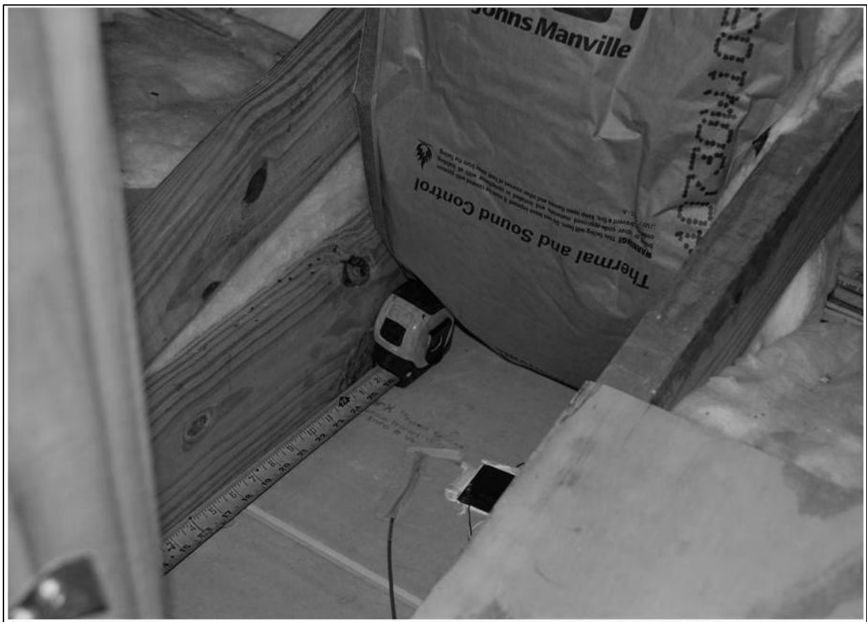
Figure 7: Heat Flux Transducer and Combo Probe Located Under Insulation
