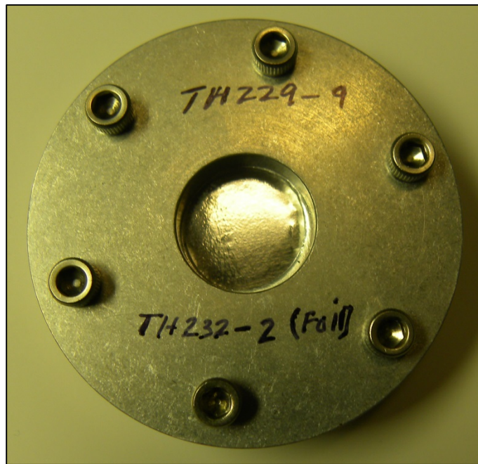
Figure 7. Packaged aluminum target holder with thorium foils inside.
