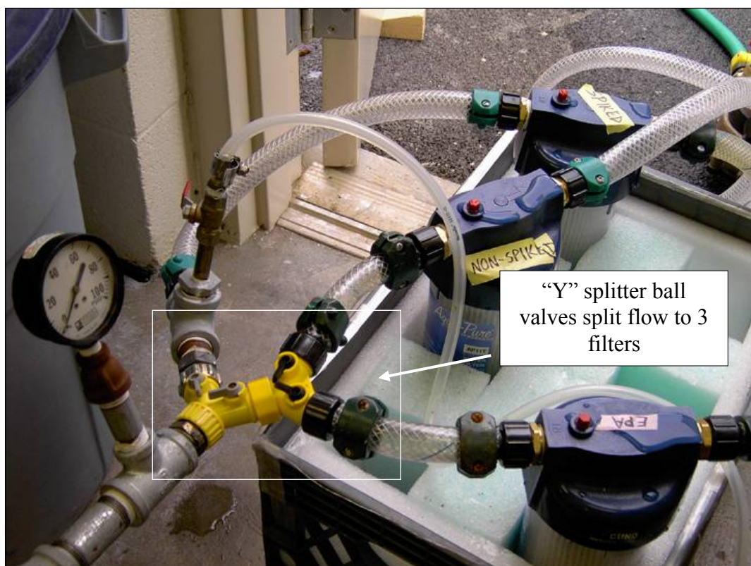
Figure 4-3. “Y” splitter ball valves were used downstream of the pressure regulator to split the flow to each filter.
