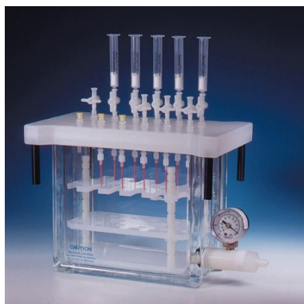
Figure 10. Twelve-port vacuum system for solid phase extraction; GL Sciences.
