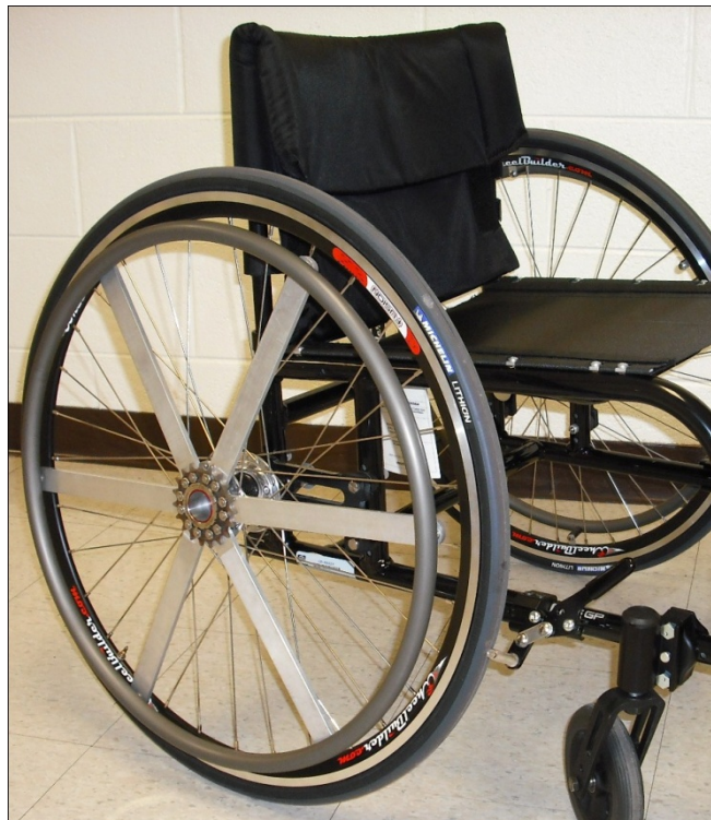
Figure 1- PowerTap hub adapted for use on a wheelchair
