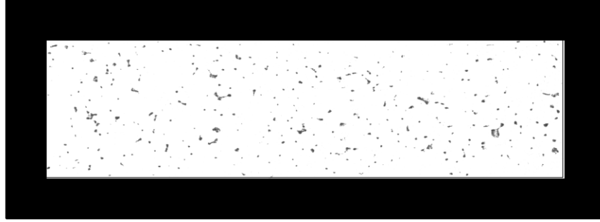
Figure 49. Inking of outer surface contact from aluminum foam annular insert
