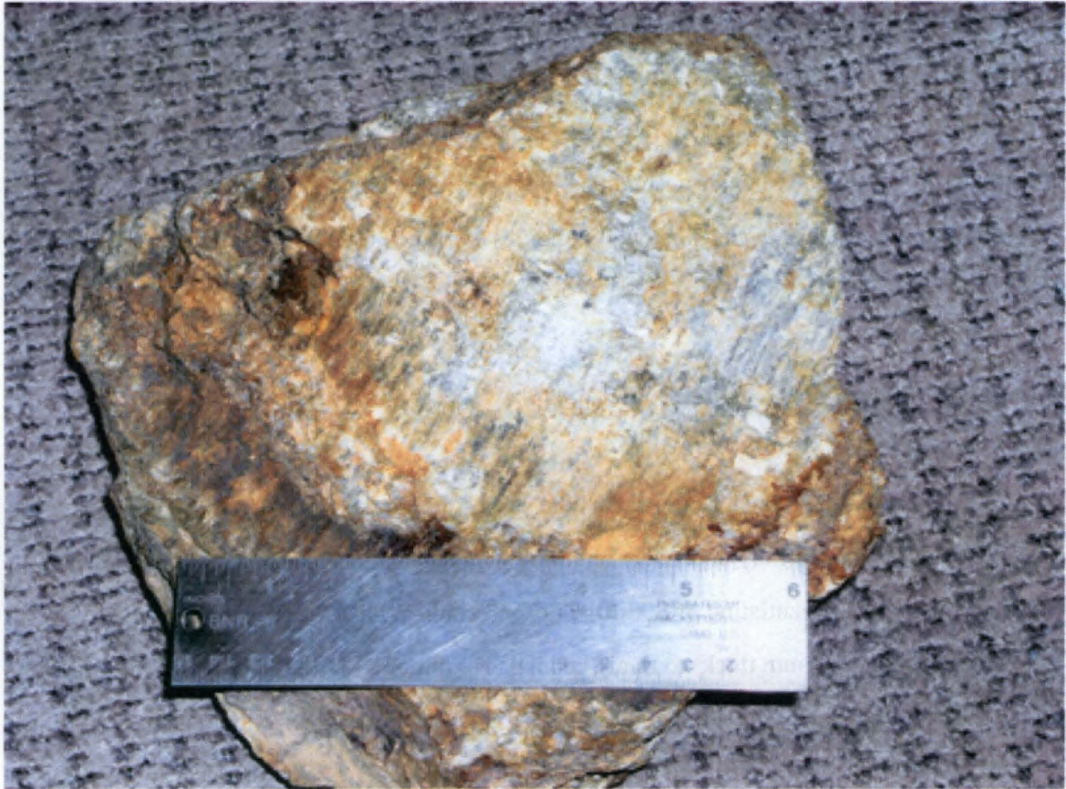
Figure 3-14. Slickenlines formed on an extremely thin graphitic bedding surface of a sample of sulfidic Dean Formation conglomerate taken from the limb of an open fold near Doublecamp Creek, Whiteoak Flats 7.5 minute quadrangle. Slickenline long axes were perpendicular or sub-perpendicular to the axis of the fold prior to removal of this sample. These lineations are most prevalent along the finer-grained surface of the a thin graphitic slate layer (almost a coating), yet not as well developed where graphitic surface is absent. It is not known whether the graphitic surface better facilitated layer parallel slip or was simply a better surface to record the occurrence of that process. Metal ruler for scale is 6 in. long.
