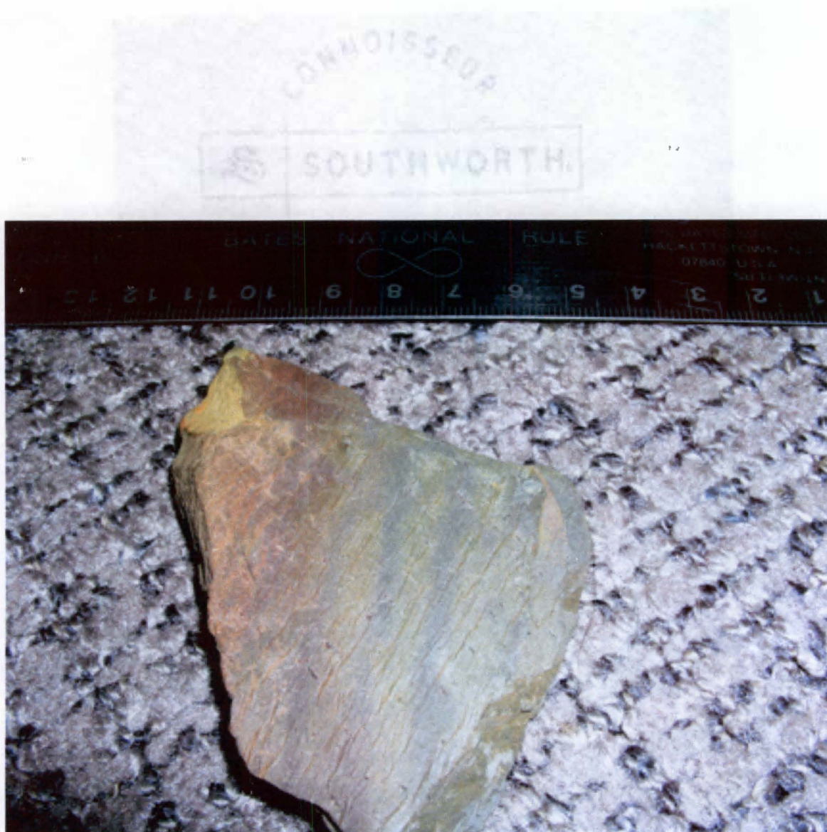
Figure 3-19. Zonal crenulation cleavage ( S_3 ) deforming slaty cleavage surface ( S_2 ) in Wilhite Formation siltstone from an exposure near Doublecamp Creek in the Greenbrier thrust sheet, Whiteoak Flats 7.5 minute quadrangle. Faint alternating light-green and dark-green stripes are bedding ( S_0 ).
