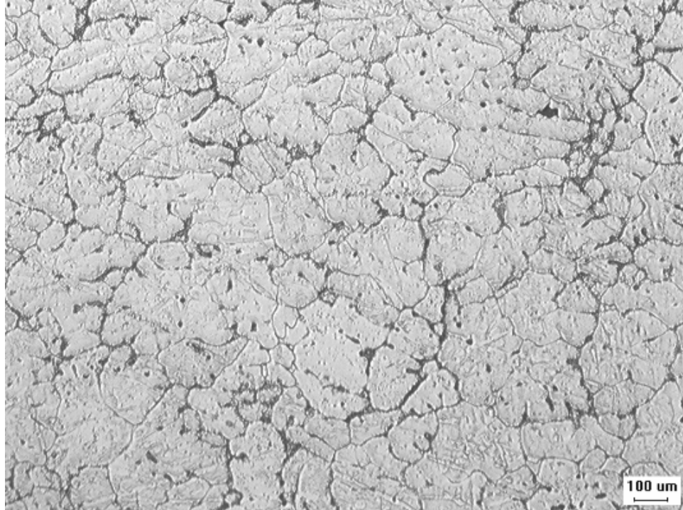
Figure 4.25: Microstructure of 6063 alloy without ultrasonic vibration at a casting temperature of 690 °C. Fully developed dendrites were obtained with average size of some millimeters.
