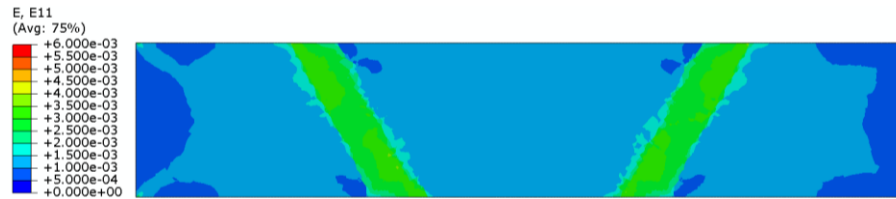
Figure 3.8 Contour plot of the strain distribution for Grade 91 steel weldment after 85 hrs creep at 70 MPa and 923K, only considering the grain size effects.
