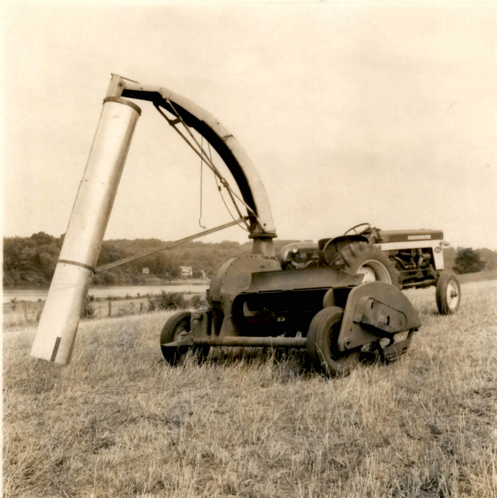
Figure 5. John Deere No. 15 flail-type forage harvester with rear baffle open.
