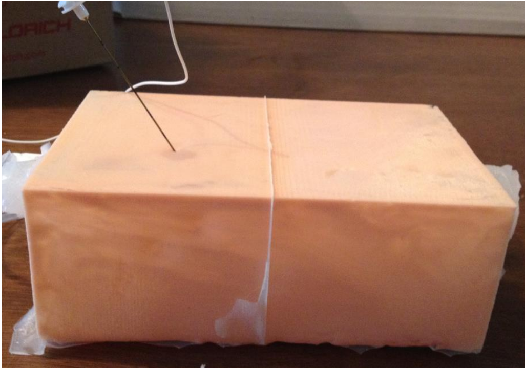
Figure 7: The needle needed to penetrate much deeper in the model before reaching the fascial plane.
