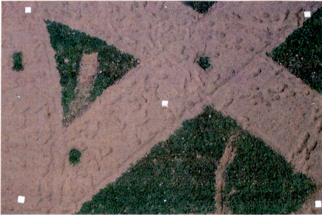
Figure 15. Block layout for the random pattern test consisted of four corner blocks and one numbered center block for geo-referencing.
