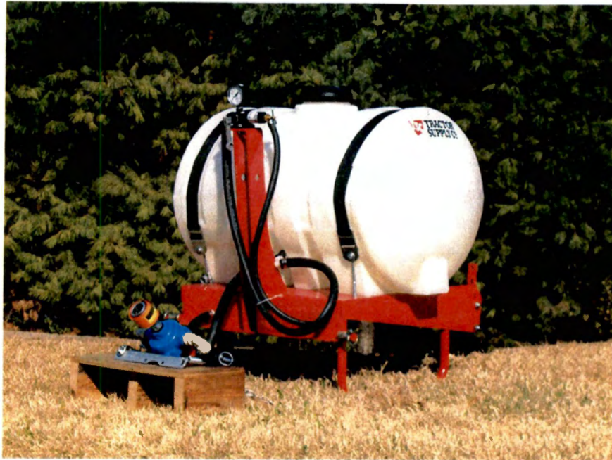
Figure 10. Sprayer and roller pump used to mount DAS and selective-type sprayer for field data acquisition.
