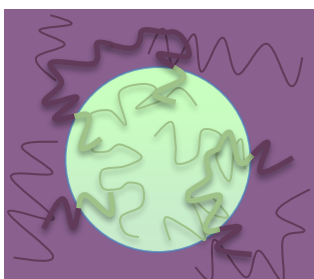
Figure 2.2. Model of compatibilizer stabilizing the interface between immiscible polymers to prevent droplet coalescence from occurring.
