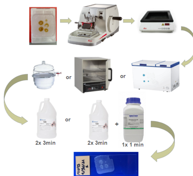
Figure 2. Step methodology of microtome, the three potential drying methods and the two potential washing methods to get a finalized slide.
