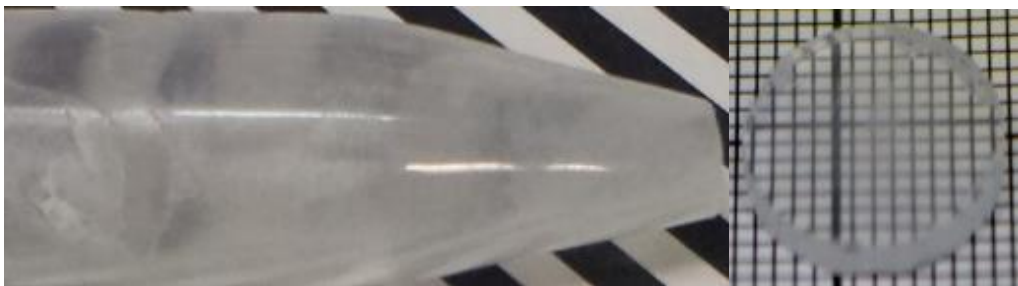
Figure 18. A 13 mm diameter single crystal boule of K 2 Sr 2 Br 5 :Eu 5% (left); a 2 mm thick polished disk (right).
