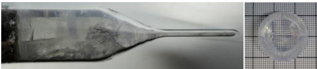
Figure 19 . A 22 mm diameter single crystal boule of \text{KSr}_2\text{Br}_5\text{:Eu 5\%} still within the quartz ampoule (left); a 10 mm tall truncated cone, \varnothing 22 mm bottom \times \varnothing 15 mm top (right). Note that despite the significantly larger size, this sample is much more transparent.
