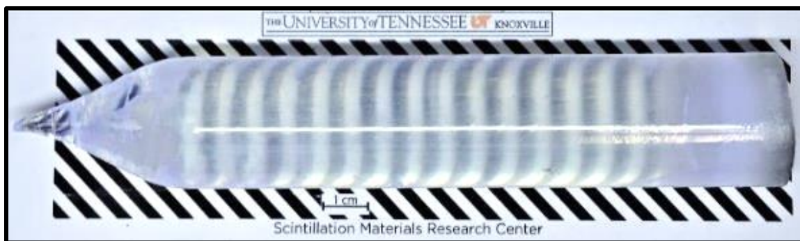
Figure 62. One inch diameter by six inch long single crystal of K 2 Sr 2 I 5 :Eu 4%, under white fluorescent light.
