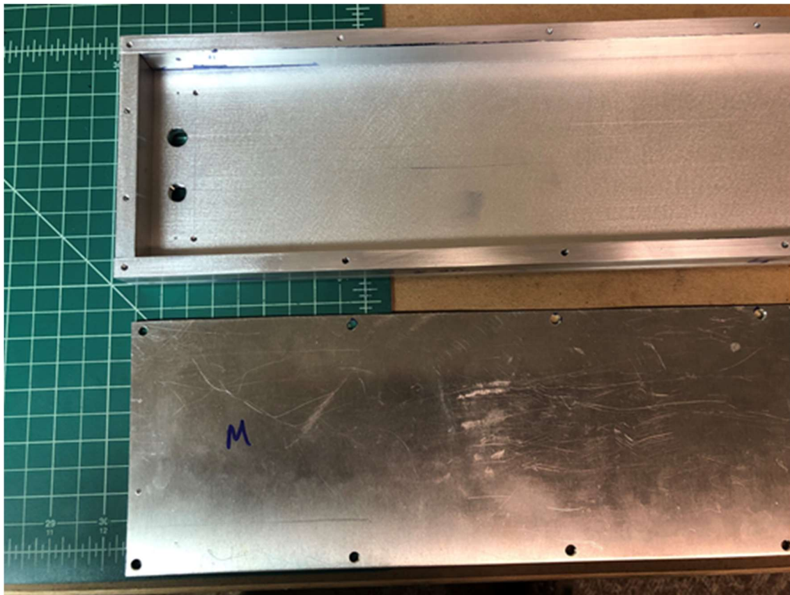
Figure 1: Test Fitting of Detector Body Components
